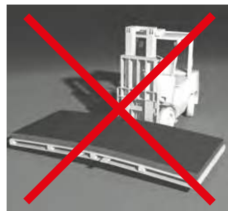
Improper forklift transport
